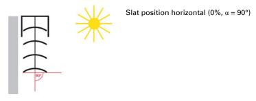
With standard blinds, the slats can be adjusted further via their horizontal position past the point where the slat adjustment ends and the blinds begin to move upwards. The slats then form an angle between 90° und 180° with the vertical.
