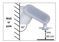
Fig. 1 The weather station must be mounted on a vertical wall (or a pole).
