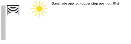
If the lower stop position is to be approached, this is specified to the blinds actuator as sun position "100%" or it will report reaching the lower stop position (i.e. sunshade fully closed) using this value. If blinds are moved down from the upper stop position, the slats first turn into an almost vertical position and the sunshade moves with closed slats to the lower stop position.
